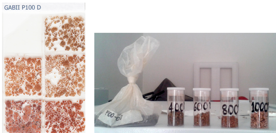
Figure 29 Left: Thin section with the soil unburnt (top right quadrant) and burnt at different temperatures. Right: the raw samples. In both cases we not the gradient in reddening.
